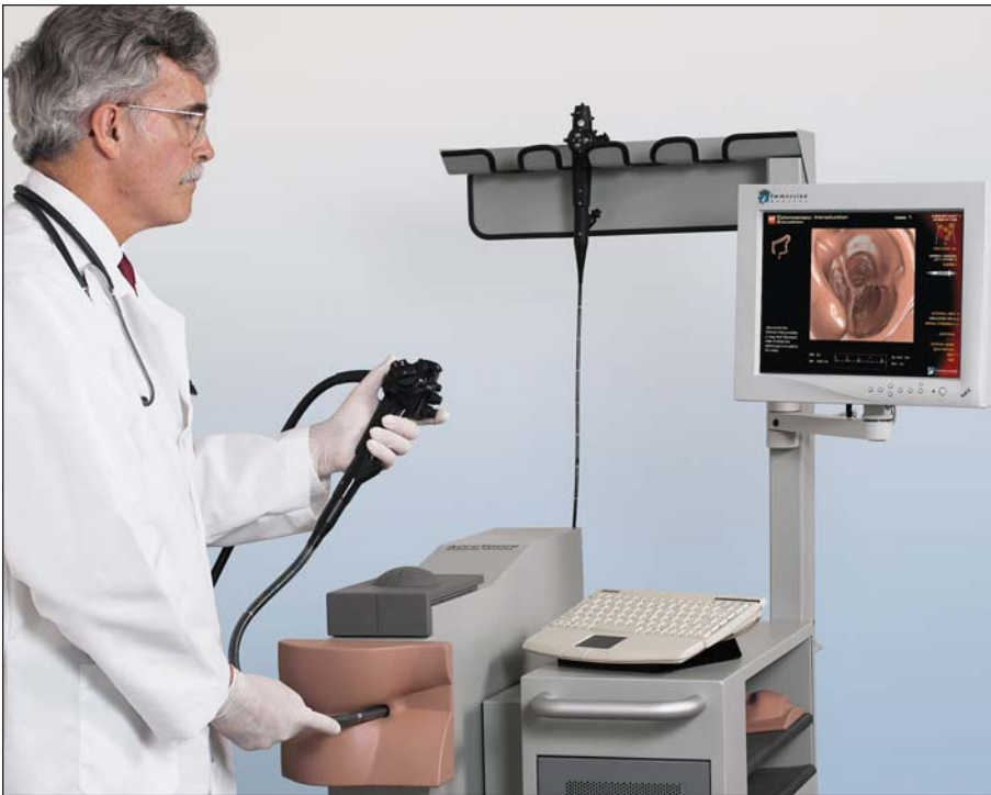
The AccuTouch system reproduces the look and feel of endoscopic procedures with realistic graphics and tactile feedback action.
