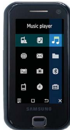
The Samsung Ultra Smart F700 is typical of the new design for mobile phones where a large touchscreen replaces a smaller display and mechanical keypad. Using haptics, interactions are immediately confirmed solving one of the central usability challenges of touchscreens.
