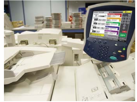
On a TouchSense-enabled touchscreen, the user perceives that buttons feel real. They seem to press and release like on a mechanical keyboard.
